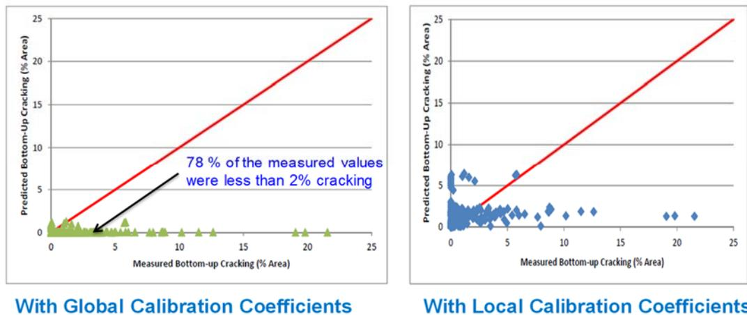
Figure 10. Virginia DOT local calibration results for flexible pavement fatigue cracking models.
