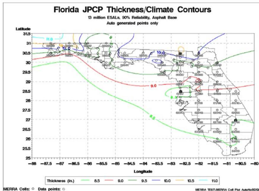
Figure 8. Florida concrete pavement thickness/climate contour map.
