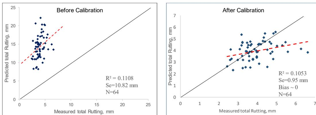
Figure 9. Ontario MOT local calibration results for flexible pavement rutting models.
