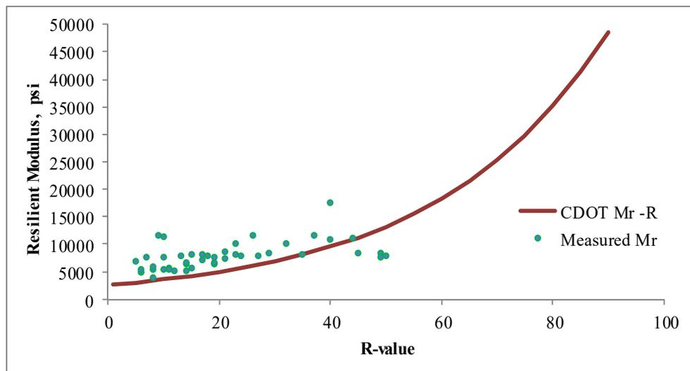
Figure 5. Colorado DOT correlation between R-value and  $M_r$  for use in Level 2 ME design.
