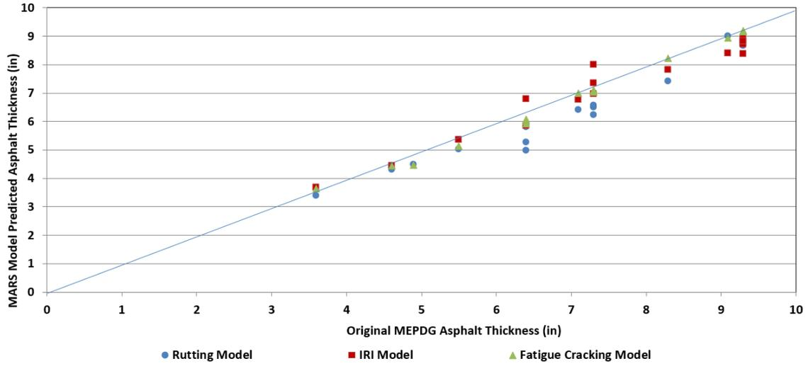
Figure 3. Comparison of HMA thickness requirements obtained using MEPDG and Kentucky design catalog.
