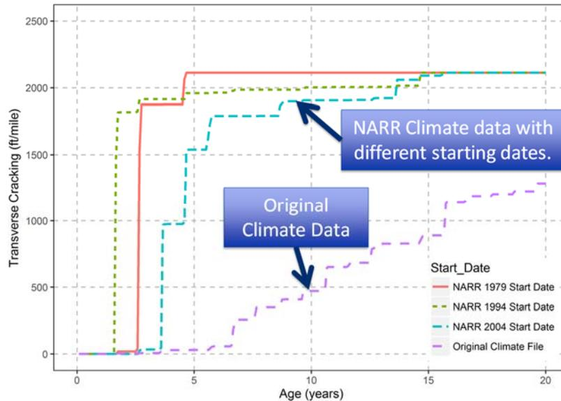
Figure 11. Effects on transverse cracking of using NCDC data and NARR data with different start dates.
