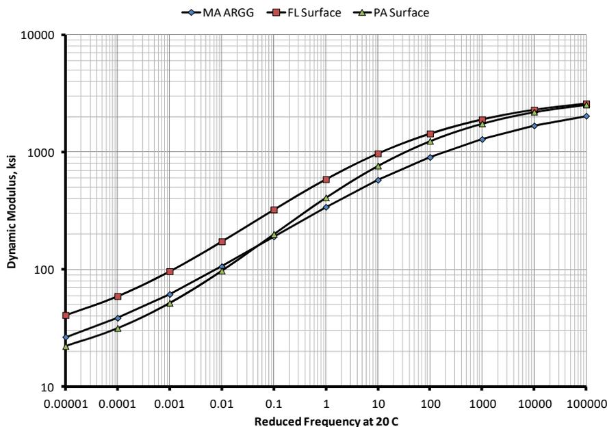
Figure 6. Dynamic modulus master curves for selected rubber-modified asphalt mixes.
