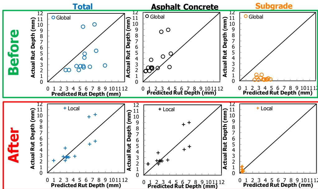
Figure 7. Indiana DOT local calibration results for flexible pavement rutting models.
