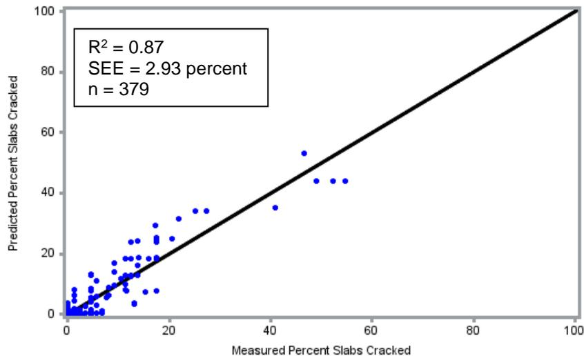
**Figure 24c. Comparison of Measured and Predicted Percentage SJPCP Overlay Slabs Longitudinally Cracked Resulting from Global Calibration Process**
