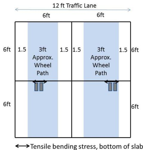
**Figure 24a. Illustration of proper location of longitudinal joints to avoid overlap with truck wheel paths (to avoid corner cracking) and the resulting critical bending stresses at bottom of slab that are considered to limit longitudinal fatigue cracking.**
