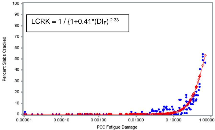
**Figure 24b. Measured longitudinal fatigue cracking (LCRK) versus PCC fatigue damage (DI<sub>F</sub>) bottom of PCC slab. [GRAPH TO BE REPLACED WITH BLACK CURVE]**
